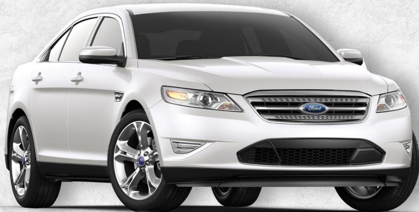
promising V8 power at close to V6 fuel efficiency. The SHO has 350 lb-ft of torque, a 6-speed SelectShift automatic with paddle shifters and all-wheel drive only.
