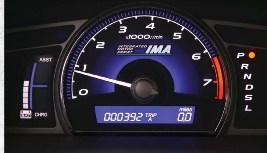
The 2006 Honda Civic has dominated the awards this year with its suite of sedans and coupes. With its unique Integrated Motor Assist (IMA) and Continuously Variable Transmission (CVT), the Hybrid is capable of 49/51 mpg city/highway making it one of the most fuel stingy cars available in the US.
