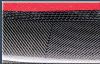
with increased aerodynamic value to the side skirt, and a carbon fiber side strike optional on the S. From the V12 Vantage comes the carbon splitter under the nose. On this, Aston Martin is quite proud to have made two angled meshes line up dead in the middle, which from a production standpoint increases the cost exponentially, they say, but in an automotive world full of carbon fiber, brings something distinctively Aston.
