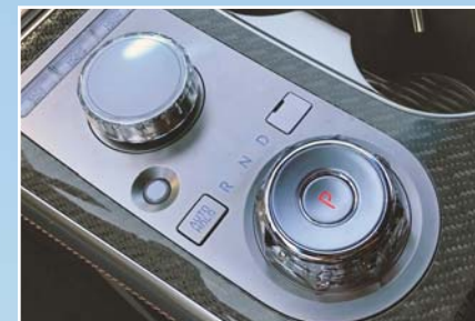
If we changed one thing on the GV70 (and its relatives), it would be this—these two dials need far better differentiation and placement, especially as one is the shifter, which should be usable eyes-off.
