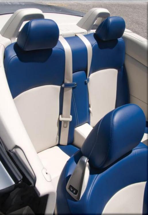
provides cup holders and storage. Rear headrests are retractable for improved visibility, with a control accessible from the rear console or from the driver's seat. Rear seat position can be shifted inboard for additional headroom. Enhanced safety features include side impact protection to mitigate the convertible structure.
