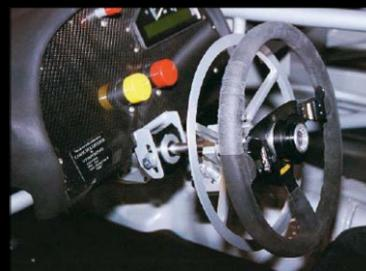
HP Motorsport of Omaha, Nebraska, constructed the Mustang for Tiger Racing and provided trackside engineering and support under the direction of Paul Brown, a veteran now in his tenth year of the World Challenge Series, and general manager for HP Motorsport. The Mustang is equipped with HPM's spec wing, SLA front suspension, Bassani Xhaust, Brembo brakes and Vortech superchargers.
